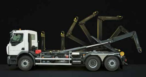
+ REMOVABLE HOOK AVAILABLE WITH MECHANICAL OR PNEUMATIC SAFETY LATCH
