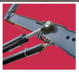
**SAFETY** Mechanical lock of main arm and tilting frame for safe tipping.
