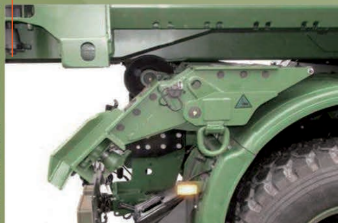
Patin de guidage stocké - twistlock arrière Rear roller support stored - Rear twistlock
